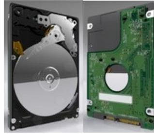
technology protects the drive mechanics and platter surfaces from shocks. WD's SecurePark™ parks the recording heads off the disk surface during spin up, spin down, and when
